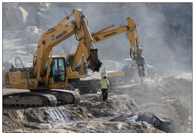
Use of hydraulic hammers to break ornamental granite rock
