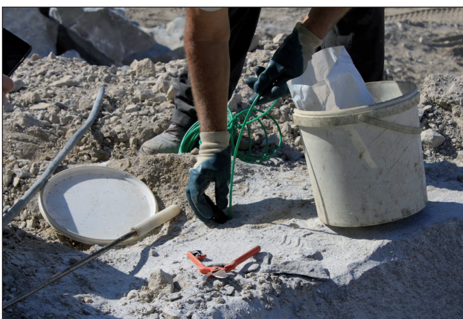
Use of Black Powder to granite extraction of ornamental rock
